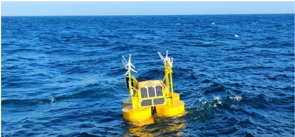
Plate 6.1: Floating LiDAR Positioned within the Bellrock WFDA
