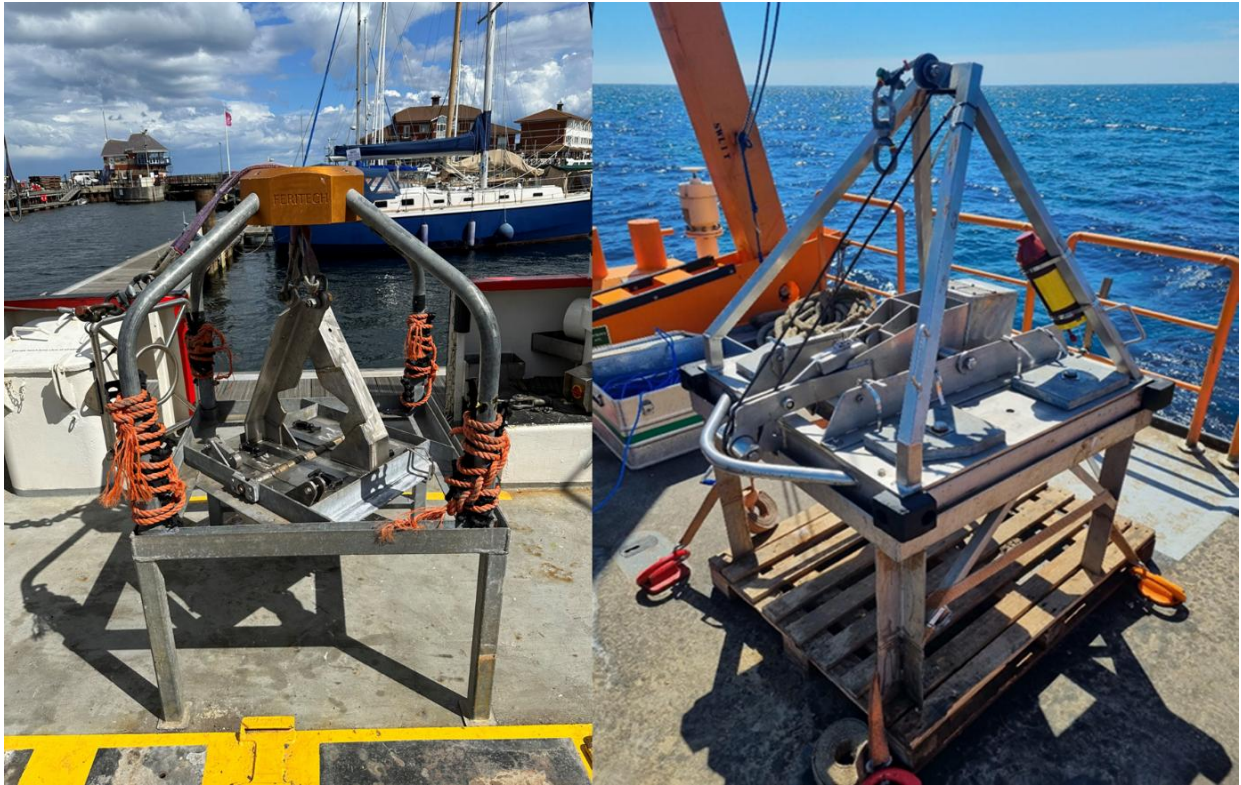
Plate 3 Left: OEL's 0.2 m 2 DVV grab sampler. Right: OEL's 0.1 m 2 mini-Hamon grab sampler.
