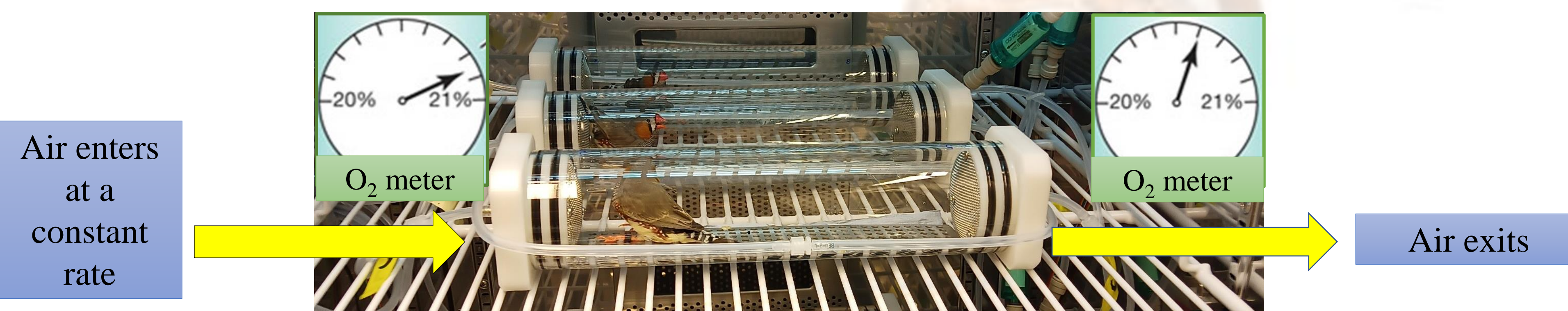
Figure 6: Schematic diagram of the principle and experimental setup of a flow-through respirometry system. Oxygen is measured before entering the chamber where the bird is kept and after exiting it, allowing estimation of whole animal oxygen consumption rate
