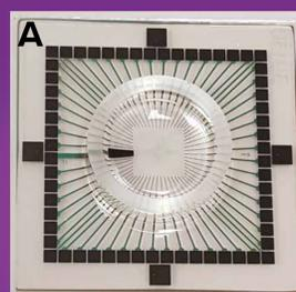
**Figure 3** (A) Commercial multielectrode array and (B) top view of recording device showing a common single ground (reference) point (black and white cables) and inputs from each side.
