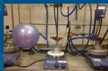
**Figure 4** A Hydrogen Isotope Exchange (HIE) reaction set up in the lab.
