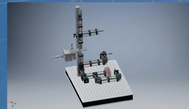
Figure 1 Schematic of our micro-spectroscopic Raman DHM system. The setup with the green central tube and green/red central tube represents the digital holographic microscope (DHM) whereas the setup with the red central tube and green/red central tube represents the Raman spectrometer.
