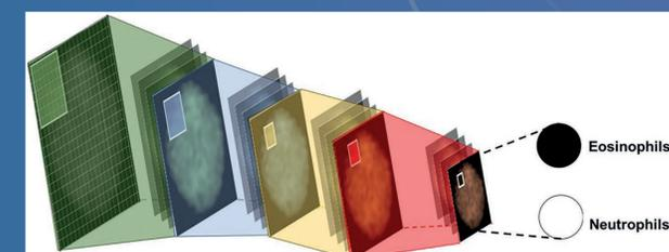
Figure 3 Schematic of a convolutional neural network to classify the DHM based phase images. Eosinophils and neutrophils are two of the different immune system cells.
