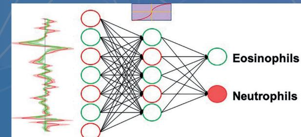
Figure 2 Schematic of a multi layered perceptron to classify the wavelength modulated Raman spectrum. Eosinophils and neutrophils are two of the different cells of the immune system.
