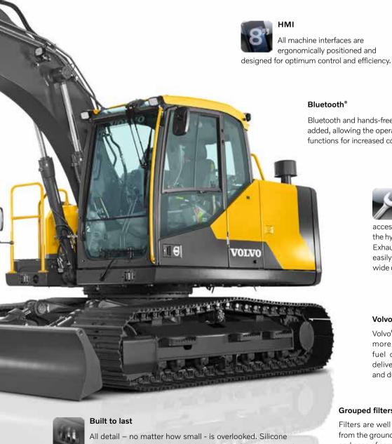
caulking is used to prevent rust, waterproof harnesses and connections have been installed - as well as heavy-duty door hinges and bolted-on protection for the framework lights.
