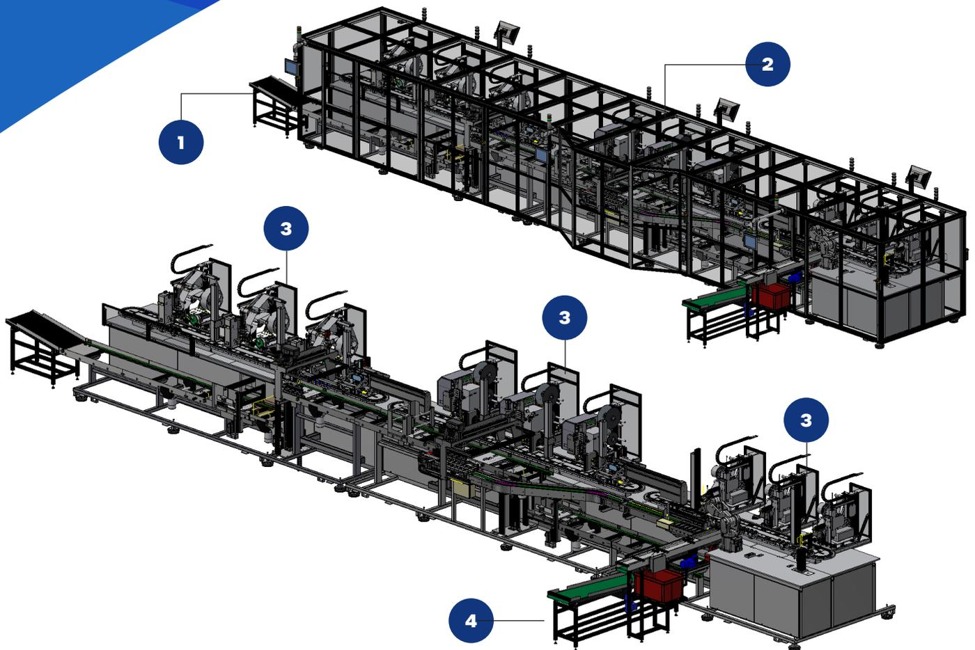
**1** Unlabelled device tray infeed and auto loading onto machine Beckhoff XTS
